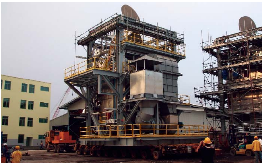
Skidded MISSION™ D-type boilers ready for delivery.
